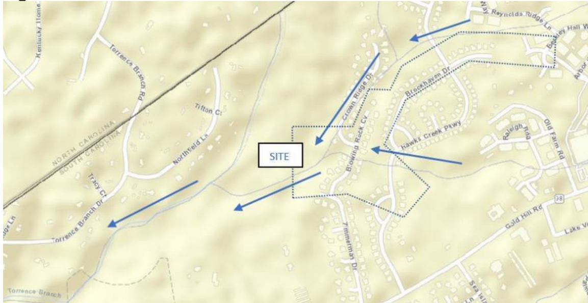
Figure 2.2: Stormwater Runoff Route
